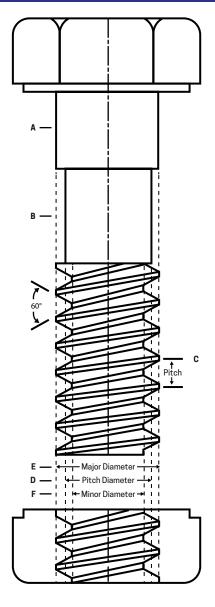
A. FULL DIAMETER SHANK: Equal to major diameter of thread. Produced by cut thread or by roll thread or extruded blank. Characteristic of machine bolts and cap screws.
